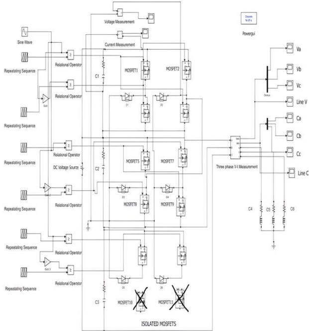
Fig. 7(a) The block diagram showcasing isolated lower arm MOSFET transistor faults of a multilevel inverter
