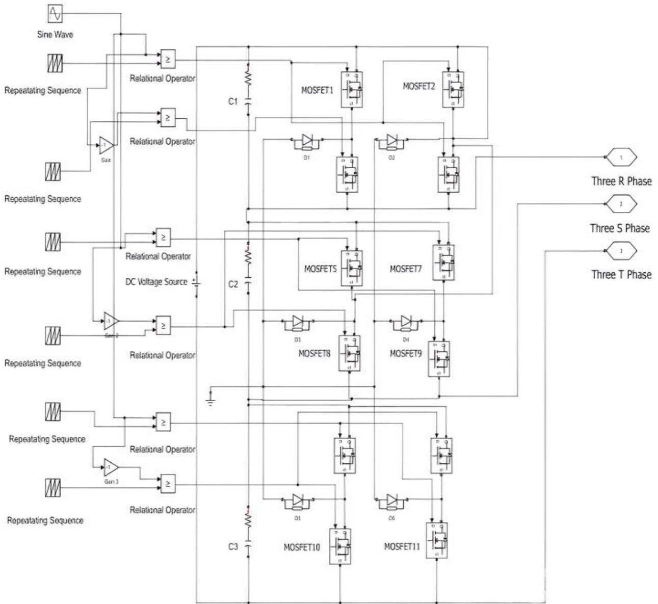
**Fig. 2 Configuration of DCMI inverter topology**
