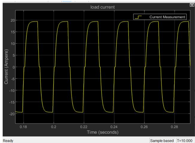
Fig. 16 Difference of Output load current when MOSFETs experience short circuit
