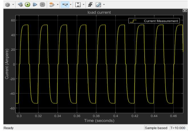
Fig. 14 Difference of Output load current under normal operating conditions
