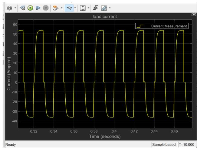
Fig. 15 Difference of Output load current when MOSFETs are isolated
