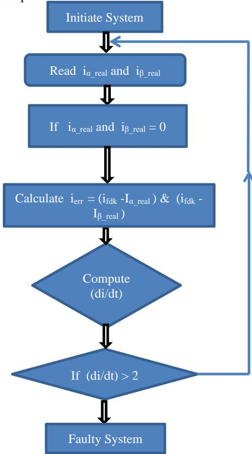
**Fig. 5 Demonstrating the use of the logic flowchart for identifying faults in the current transducer**
