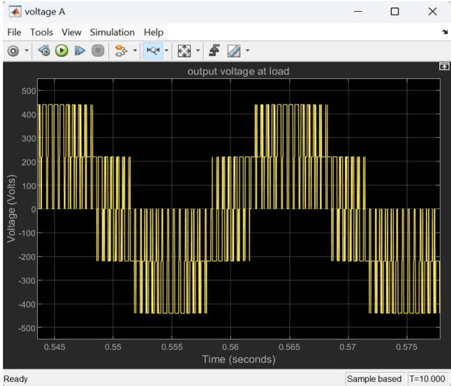
**Fig. 8** Output voltage signal functioning under normal operating conditions supplying an R-L load
