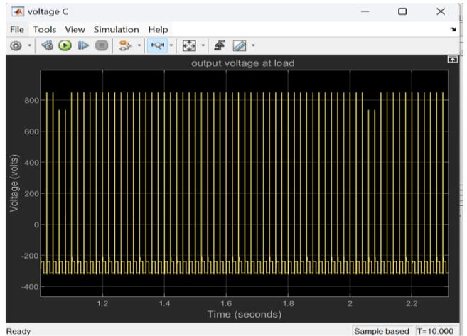
**Fig. 10** Output voltage signal when the lower arm MOSFETs are in a short circuit supplying R-L load
