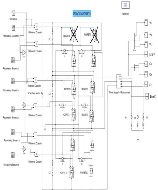
Fig. 7(c) The block diagram showcasing isolated upper arm MOSFET transistor faults of a multilevel inverter
