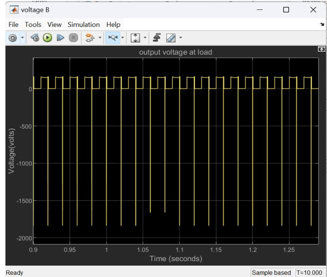
**Fig. 9** Output voltage when lower arm MOSFETs are isolated in an R-L load configuration
