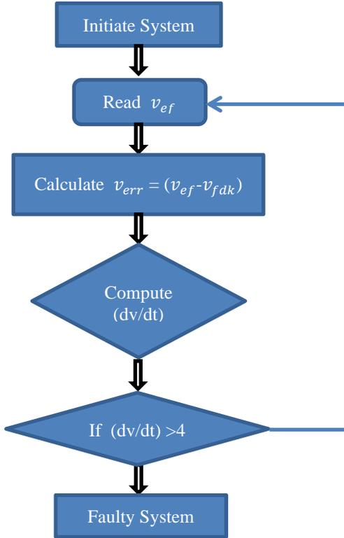
Fig. 4 Demonstrating the use of the logic flowchart for detecting faults in the speed transducer
