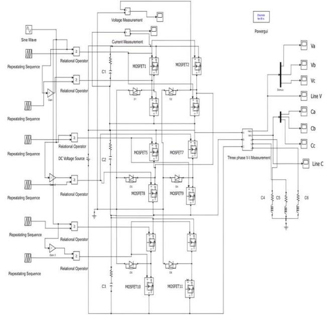
**Fig. 6 Simulation circuit diagram for a multilevel inverter supplying an (R-L) load**
