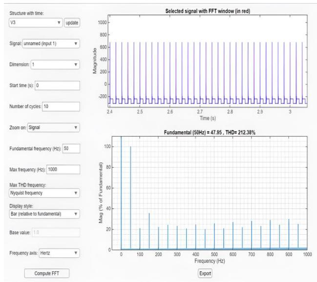
**Fig. 13(c)** The lower arm MOSFETs are short-circuited
