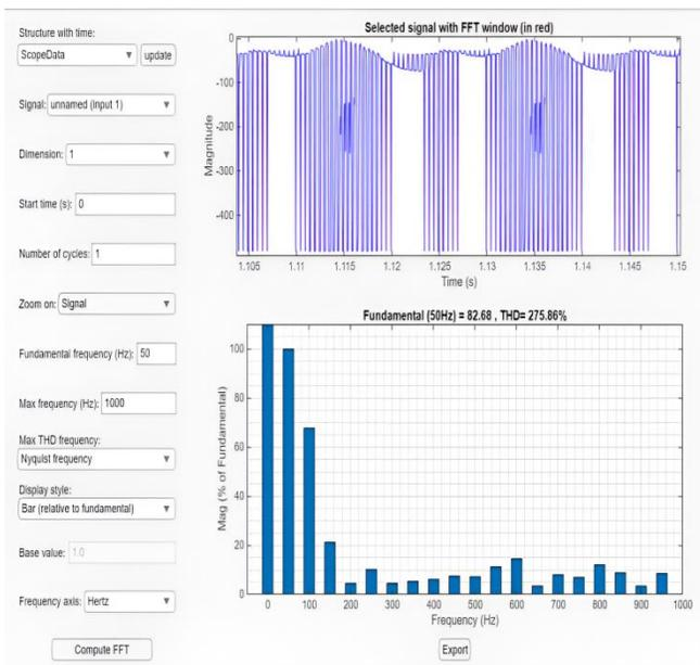
Fig. 13(e) The upper arm MOSFETs are short-circuited
