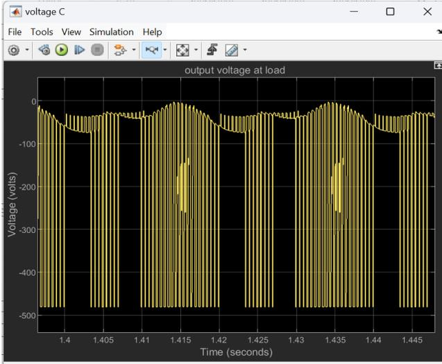
**Fig. 12** Output voltage signal when the upper arm MOSFETs are short-circuited in an R-L load
