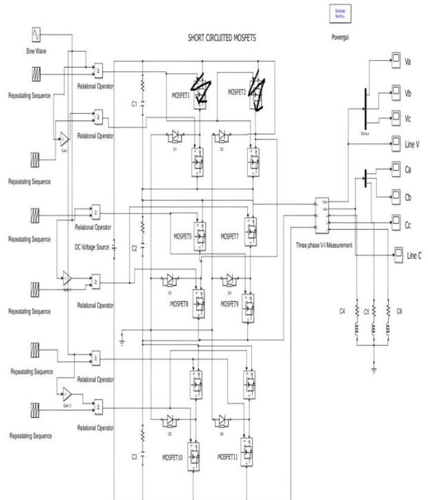
Fig. 7(d) The block diagram showcasing short-circuited upper arm MOSFET transistor faults of a multilevel inverter
