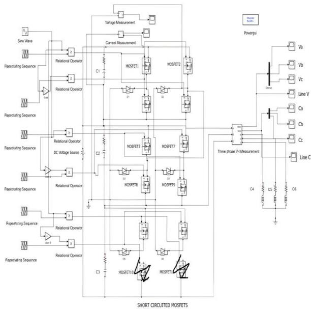
Fig. 7(b) The block diagram showcasing short-circuited lower arm MOSFET transistor faults of a multilevel inverter
