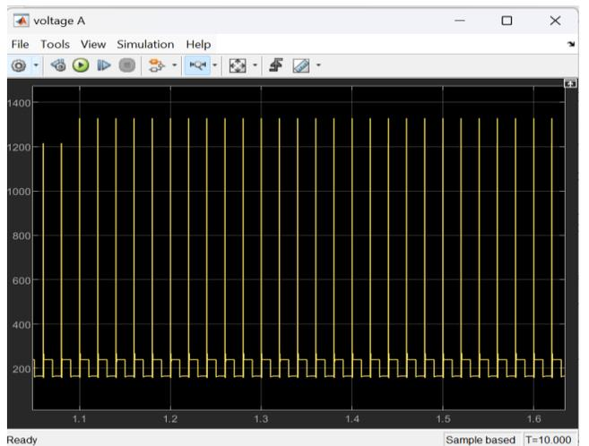
**Fig. 11** Output voltage signal when the upper arm MOSFETs are isolated in an R-L load
