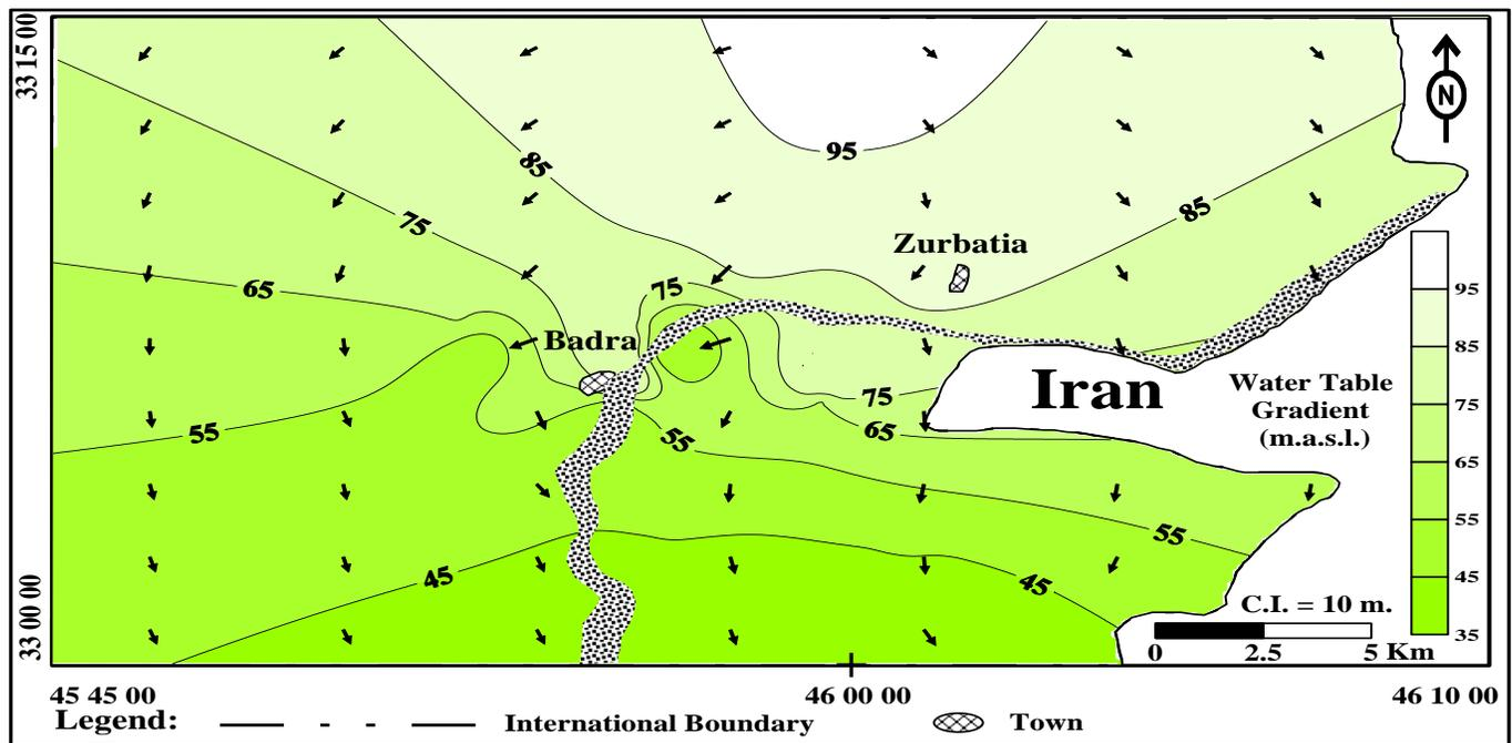
Fig. 6 Flow net map of groundwater in the unconfined aquifer
