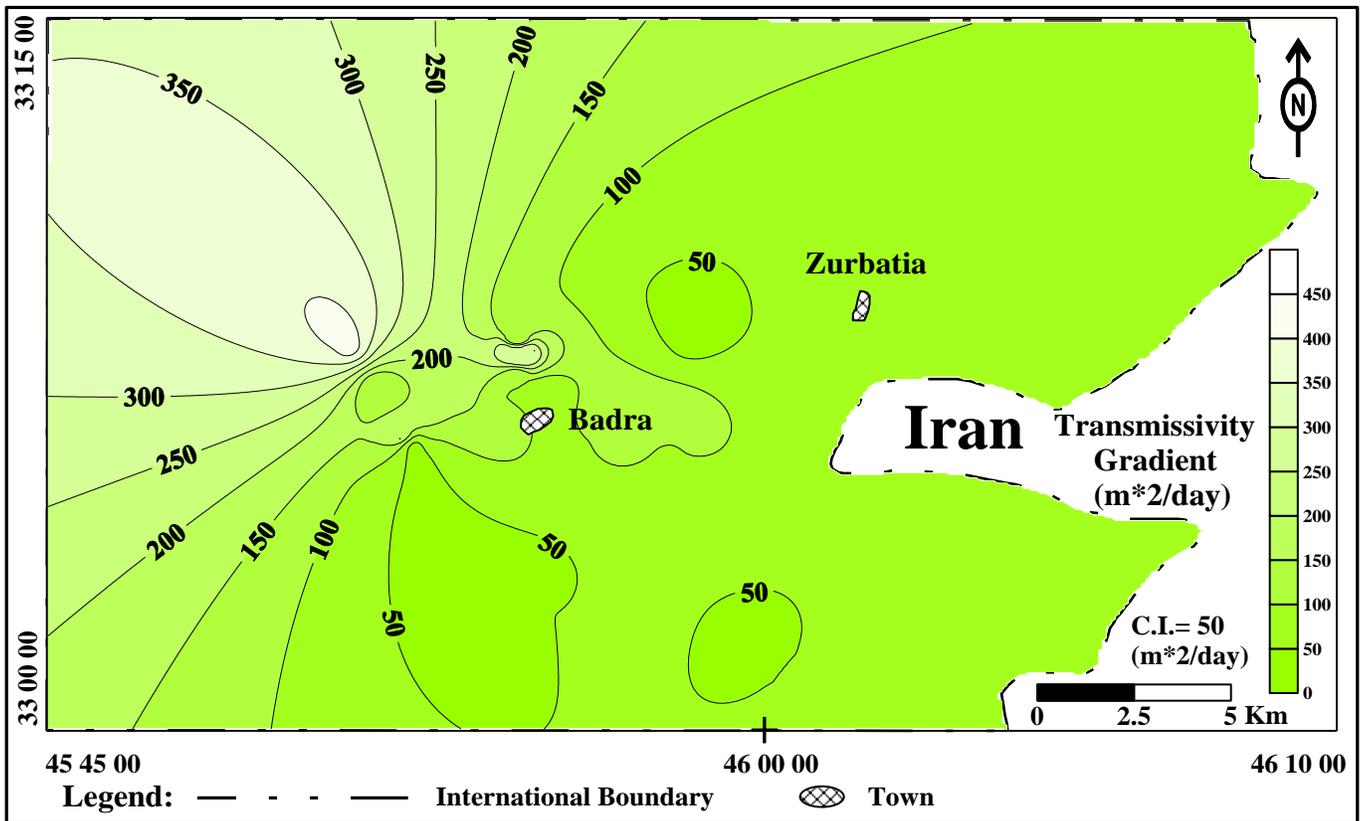
Fig. 4 Transmissivity map of the unconfined aquifer
